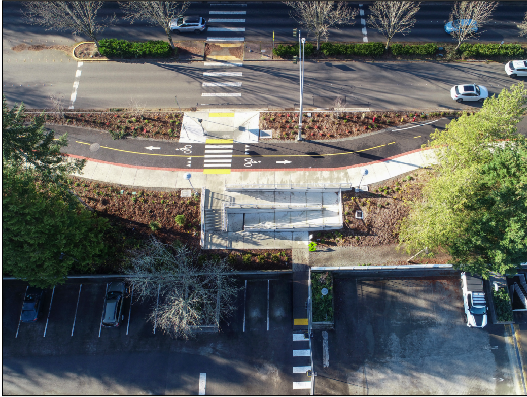
Cycle Track ADA ramp connection to Microsoft garage
