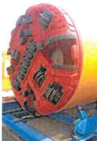
We will use microtunneling to cross under the Sammamish River.
