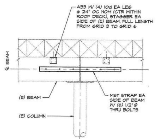
ABS W/ (4) 10d EA LEG @ 24" OC NOM (CTR WITHIN ROOF DECK), STAGGER EA SIDE OF (E) BEAM, FULL LENGTH FROM GRID 3 TO GRID 6
