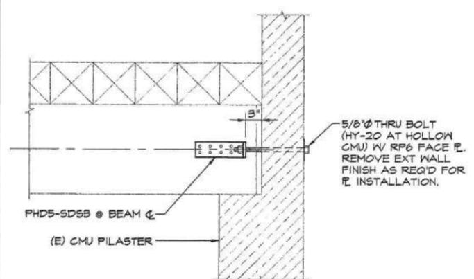
5/8" THRU BOLT (HY-20 AT HOLLOW CMU) W/ RP6 FACE FL. REMOVE EXT WALL FINISH AS REQD FOR FL INSTALLATION.
