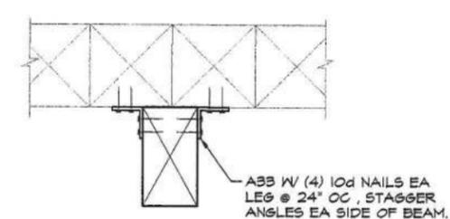
ABS W/ (4) 10d NAILS EA LEG @ 24" OC, STAGGER ANGLES EA SIDE OF BEAM.
