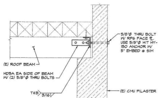
5/8" THRU BOLT W/ RP6 FACE FL. USE 5/8" HIT HY-150 ANCHOR W/ 5" EMBED @ SIM
