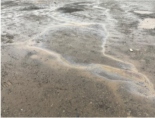
Photograph 7. Sheen on gravel parking lot on the western portion of the Property.
