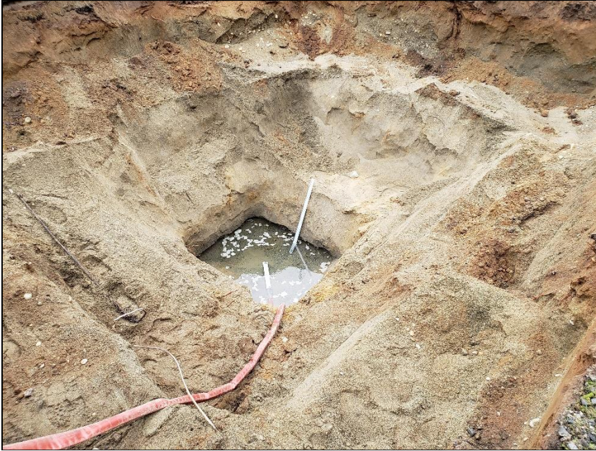
Plate 3: View of infiltration testing at PIT-1 underway.
