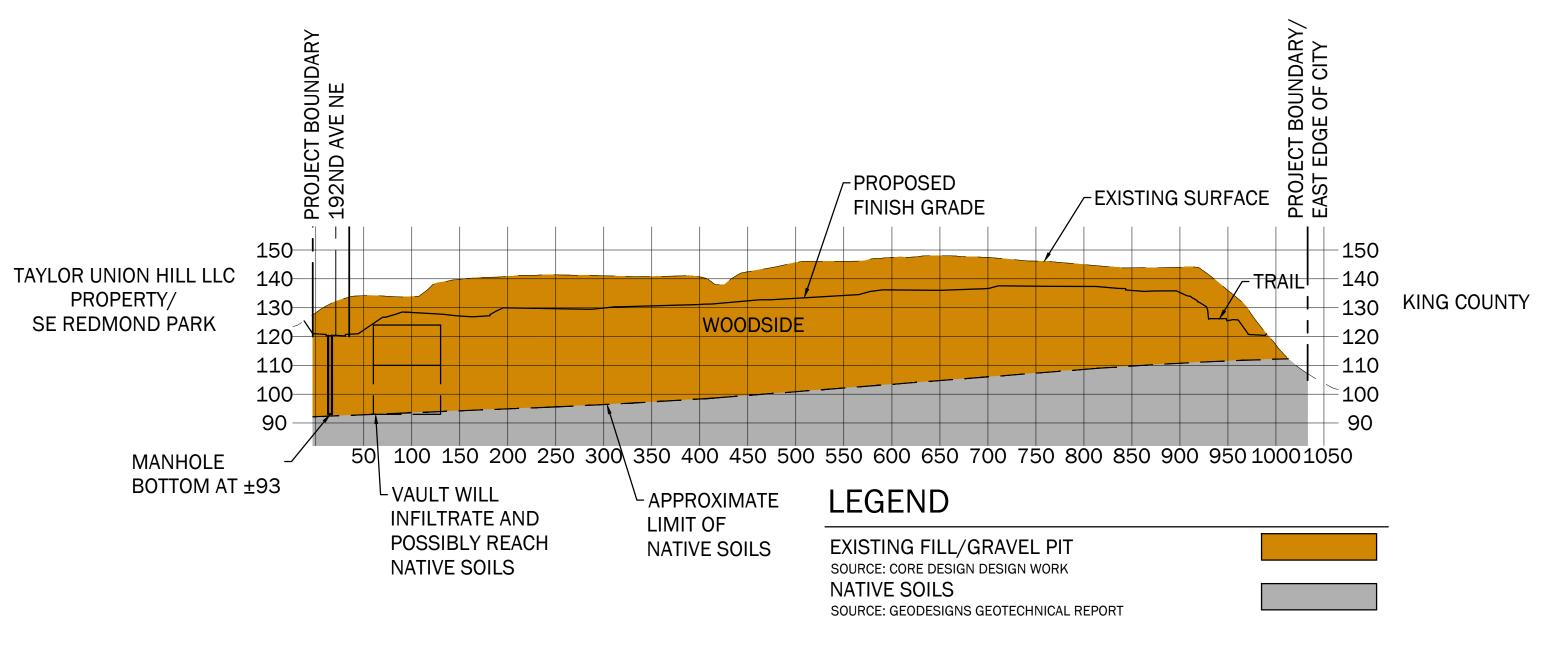
NOTE: THIS EXHIBIT SHOWS THE APPROXIMATE LIMIT OF NATIVE SOILS WITH THE PROPOSED DEEPEST UTILITIES (VAULT AND MANHOLE IN ROUNDABOUT AT 192ND AVE NE AND NE 70TH ST). THE REBUILDING OF THE SLOPE ON IS CLOSE TO NATIVE SOILS. SEE GEOTECH REPORT FOR DETAILS.
